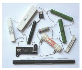
power. A wound component may have a small inductive component, and designers are sometimes exhorted to use non-inductive types like the bifilar-wound Mills or Mundorfs; however, as seen in the test values, the inductance was essentially negligible.
